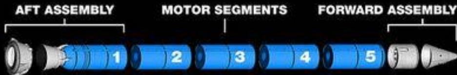
Stacking begins with the **AFT ASSEMBLY** at the Rotation, Processing and Surge Facility at Kennedy Space Center.
