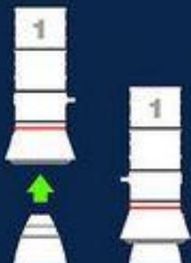
**AFT EXIT CONES** are then stacked with their nozzles to form **AFT ASSEMBLIES**.
